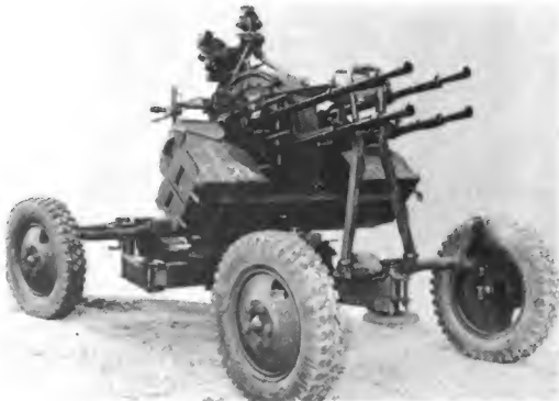
Figure 6-46. 14.5-mm ZPU-4. This four-barrel anti-aircraft machinegun mounted on a towed four-wheel carriage is used in many motorized rifle regiments. The 14.5-mm machinegun also appears in double and single mounts.
